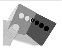
Gently heat up the back of the overlay with the hair dryer.
