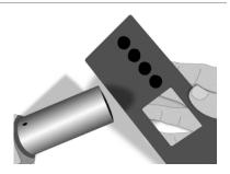
Then, also heat up the surface of the keypad with the hair dryer.
