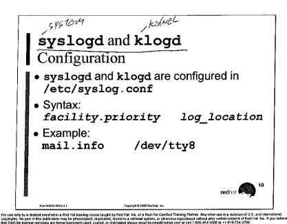
The standard system logging daemons syslogd and klogd are both configured with /etc/syslog.conf. It is possible to configure what kind and what amount of system messages is stored in specific log files.
