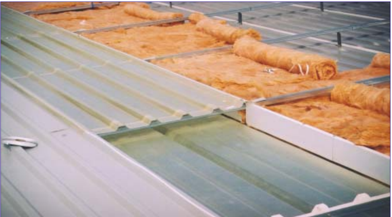
Filon Fermacore fitted over Filon Liners (unseen), with Filon SupasaFe outer skin fitted over the Three Skin Assembly
