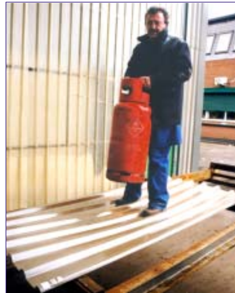
FILON SupasaFe Without Fixings Supports a Person Carrying a Heavy Load
