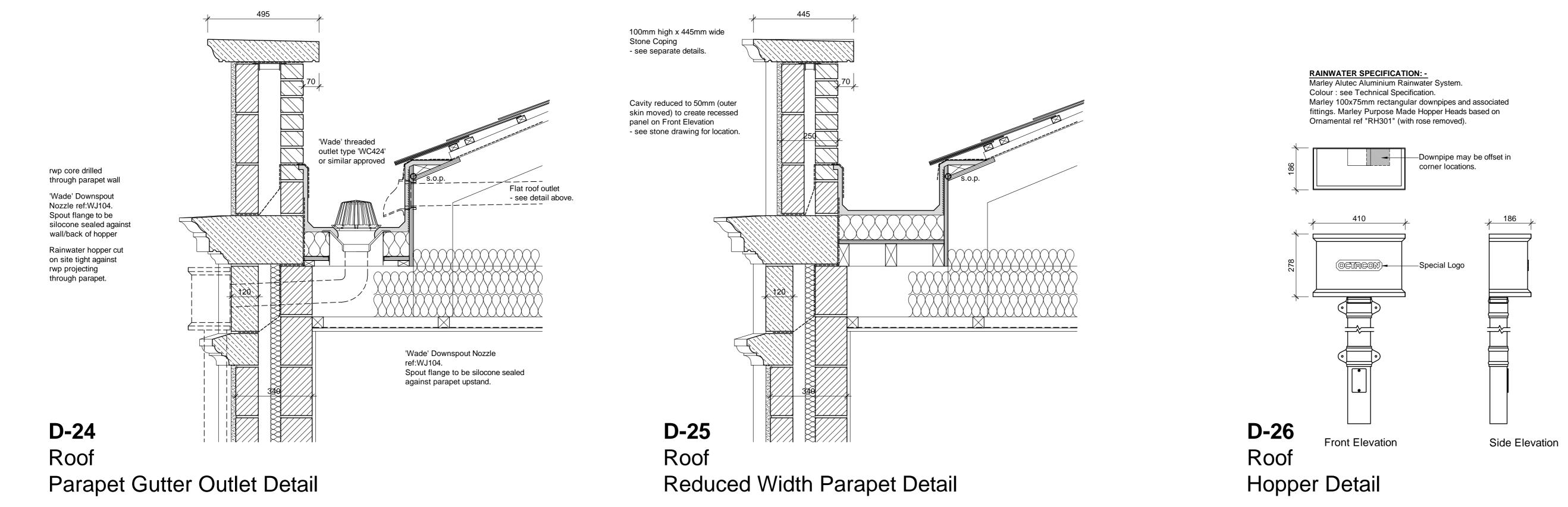
Parapet / Back Gutter Detail
