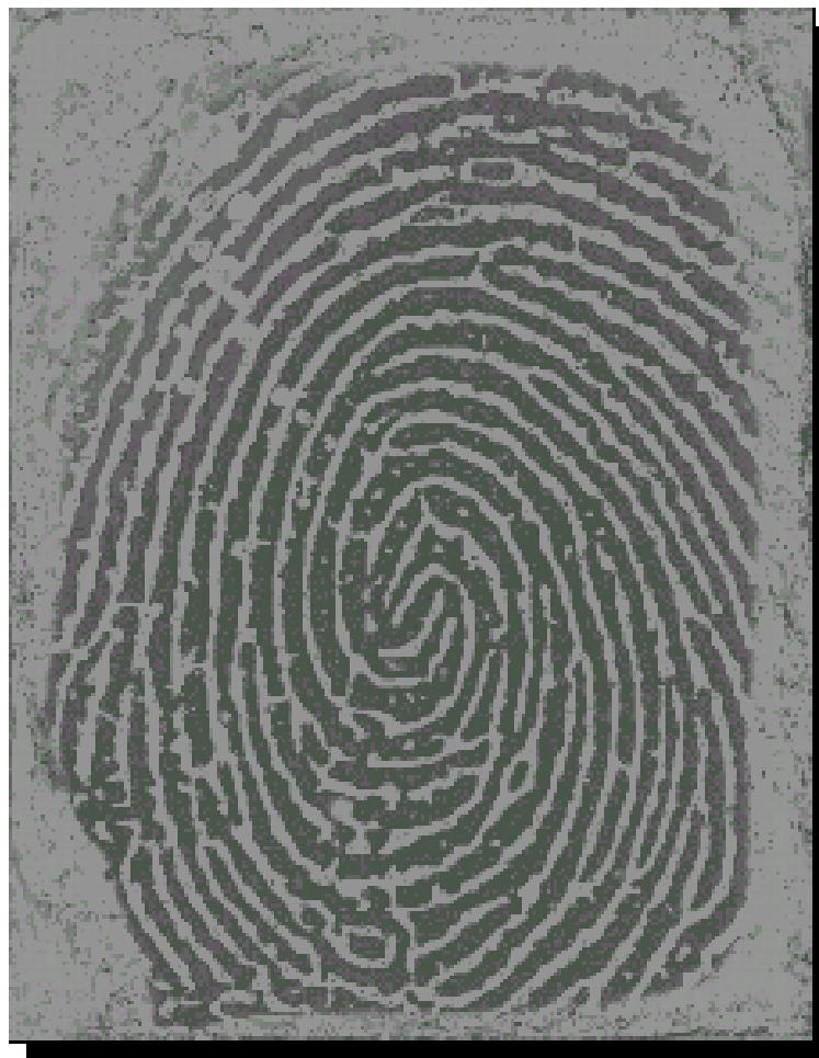
Captured Fingerprint Image of the Gummy Finger with the device H (a capacitive sensor)
