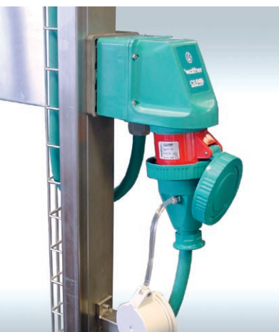
Only one connecting cable between automatic caustic soda applicator and loader
