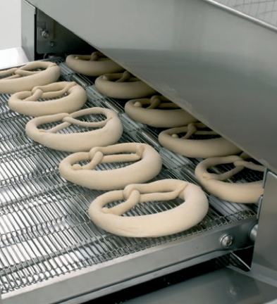
Causted soda shower with two additional causted soda curtains
