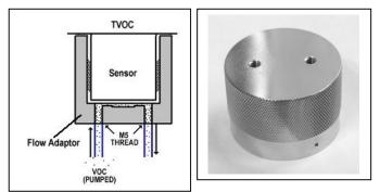
If a unit is to be placed in an inaccessible or difficult to reach location TVOC can be fitted with a Fixed bump adaptor, part number 849217 to enable remote bump testing. This enables the unit to work as a diffusive instrument but allows a bump gas to be applied. This again would replace the standard sensor cap and looks as follows:
