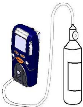
Figure 4.1 Bump Test / Gas calibration set up
