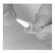
Warning: Use caution when handling α-alumina powder. Do not inhale powder. Avoid contact with skin and clothes. Wash hands thoroughly before eating, drinking, smoking or applying cosmetics. The powder contains a TVL(TWA) of 10 mg/m<sup>3</sup>.
