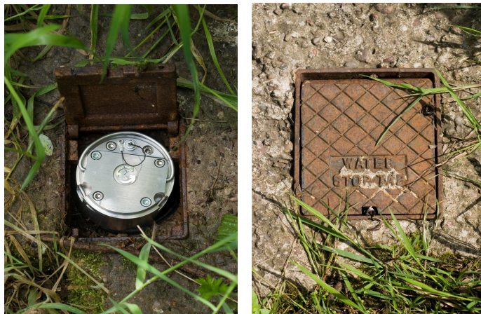
Figure 2. The GasClam® fits in to a standard borehole making it safe and secure on site.
