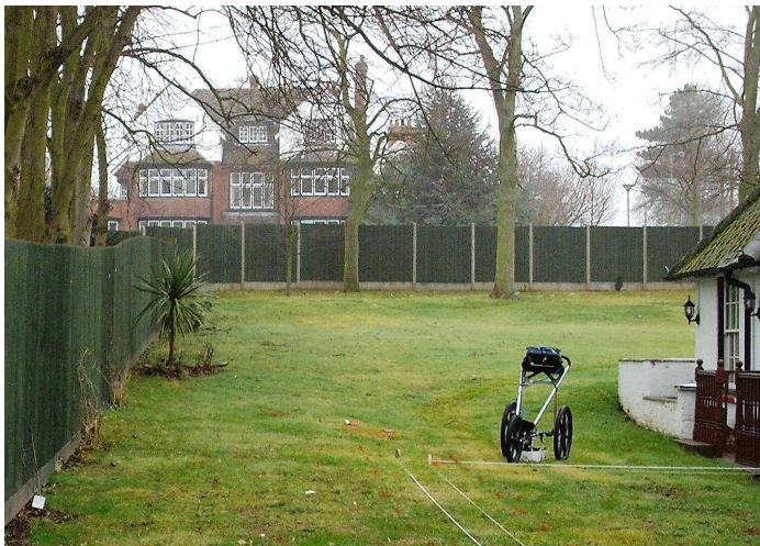
GPR for locating tree roots using automated trolley
